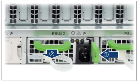
Figure 19: Unlocking and removing the power supply unit
